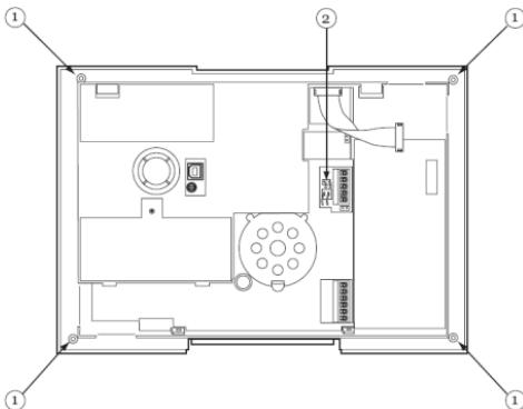
5. Before completely removing the rear housing panel, lift it slightly and pull out the siren plug.
